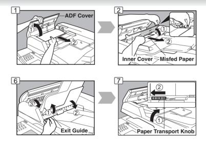
Removing a Misfed Paper (System Console)
